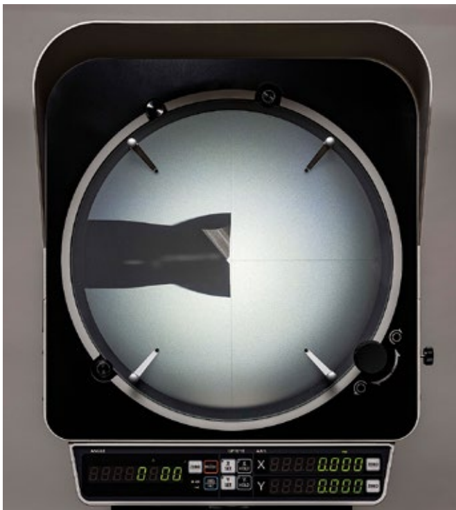
Example of attaching the LED circular illuminator on PJ-PLUS
