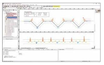
Example of contour-tolerancing result displayed graphically.
