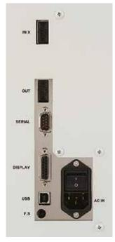
The HR-530 provides a variety of interfaces for convenient data transmission.
