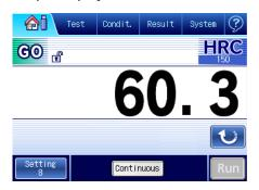
Only displays test result and scale, appropriate for repeated testing under the same conditions.
