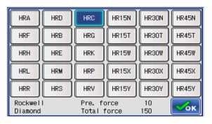
Directly select the required hardness scale from the menu and have full control over the time cycle settings.
